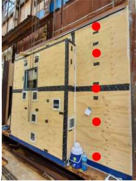
*Figure 2: Node locations (1-5 from bottom to top)*
