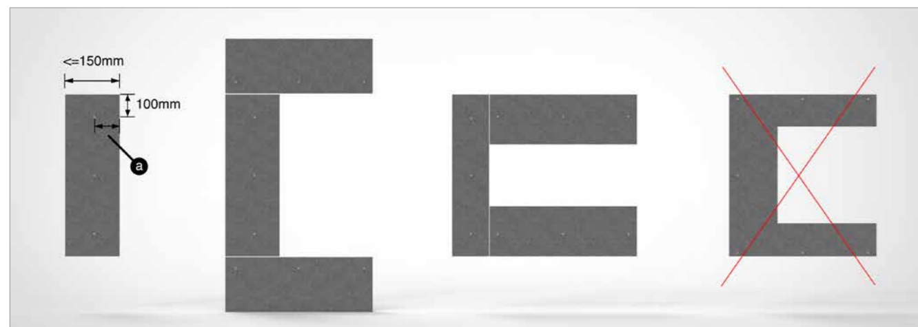
FIGURE 21. Correct installation of Genesis façade boards at windows, doors and openings a: If the small cut-outs are not wider than 150mm, they can be mounted with only one rivet in the middle of the board.
