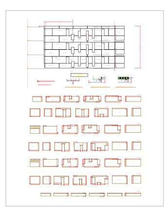
Example of CAD drawing supplied by customer as a .dwg file at 100%. Top shows the entire wall allowing for doors and windows.
