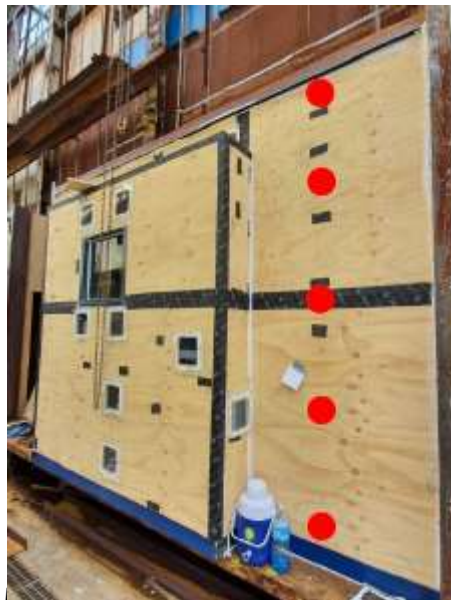
Figure 2: Node locations (1-5 from bottom to top)
