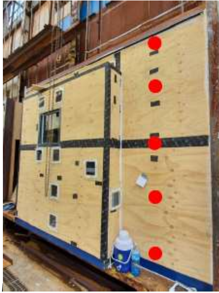
Figure 2: Node locations (1-5 from bottom to top)
