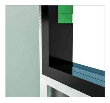
5. APPLYING THE TAPE TO SILL Repeat this process for the rear edge of the frame, then do the right a left hand side and finish off with the header.
